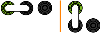
Figure 5. Wall socket earth applied
